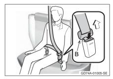
2 To release the hooked plate "A", insert the plate "B" or the mechanical key (→P. 3-1) into the hole on the buckle.
