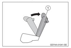
Raise the head restraint\* to the highest position. If the head restraint interferes with the child restraint system and it cannot be installed correctly, remove the head restraint. (→P. 3-35)
