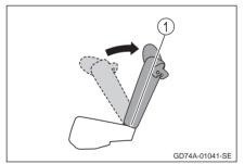
2 Raise the head restraint\* to the upper position. If the head restraint interferes with the child restraint system and the child restraint system cannot be installed correctly, remove the head restraint. (→P. 3-35)
